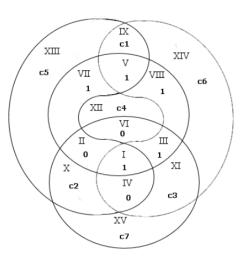
c. To make this a well-defined binary linear code, number the 8 regions where an odd number (1 or 3) of A, B, C or D overlap I, II, III, IV, V, VI, VII, VIII – as shown at right and consider these the digits
