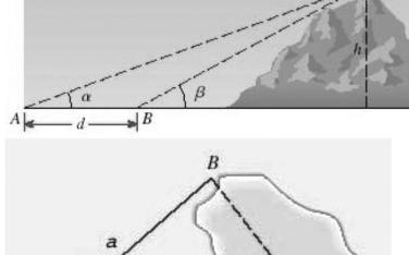
9. To find the distance across a lake, a surveyor has taken the measurements a = 11 mi., b = 13 mi. and  $\angle C = 40^{\circ}$ . Find the distance across the lake using this information. Round to 2 significant digits.
